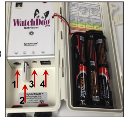
Figure 1 - Retriever External Ports
