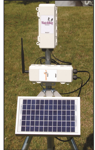
Figure 15 - Retriever and DataScout setup with solar panel
